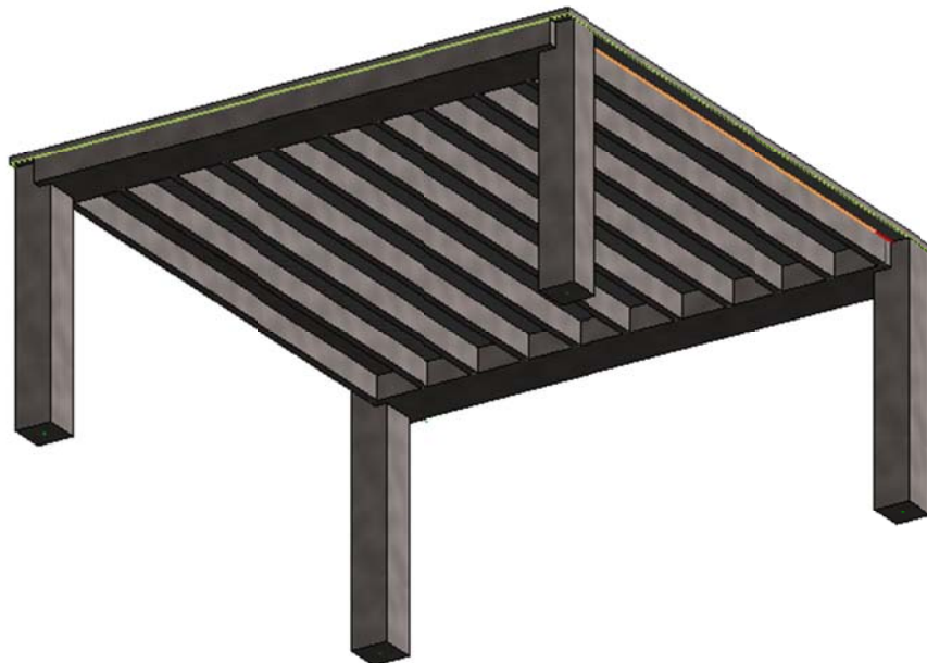
Figure 15 Typical bay layout for One-Way Pan Joist and Beam (30'-0" by 30'-0" between column lines K'-L' and 3'-4') (Modeled in Revit Structure)
